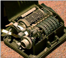
HAGELIN M-209 CIPHER MACHINE (GVG / PD)
